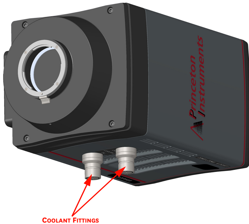
Figure C-1: Positioning Sophia 4096B to Drain Coolant
